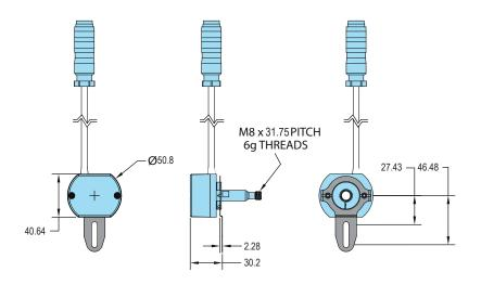
All dimensions are in mm with a tolerance of ±0.127mm or ±0.254 unless otherwise specified
