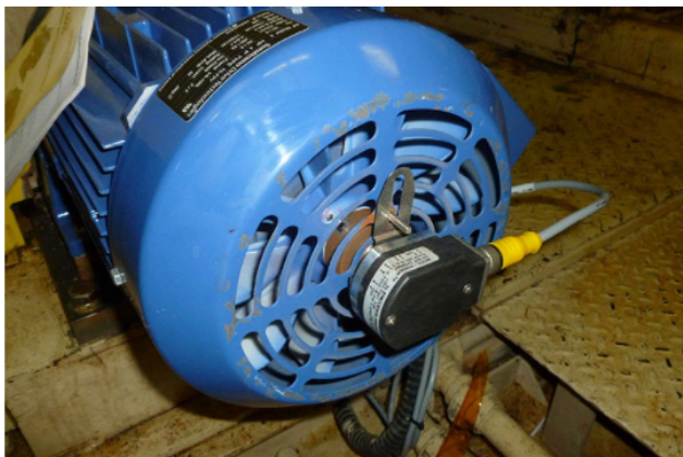
a compact, 2-inch blind hollow bore encoder (1) provides motion feedback on a motor. The flex mount (2) stabilizes the encoder, and the cable sends the electrical signal to the receiver.
