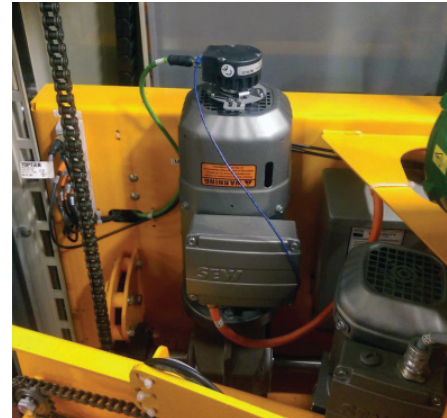
Model 25H encoder mounted on a motor
