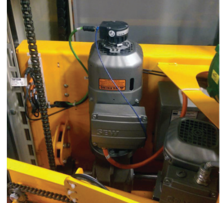
Model 25H encoder mounted on a motor
