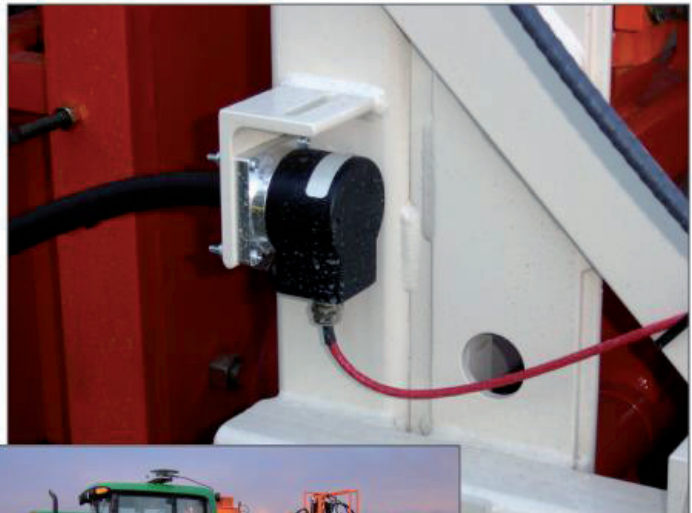
Flexible shaft-mounted Model 702 installed on agricultural harvesting equipment
