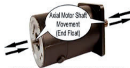
Figure 2 - Axial Movement of a Servo Motor
