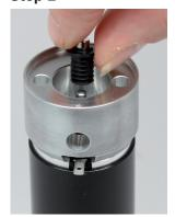
Install Magnet Holder, with magnet in place, over motor's shaft.
