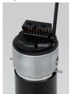
Install 30M Encoder Module on adapter with mounting screws.
