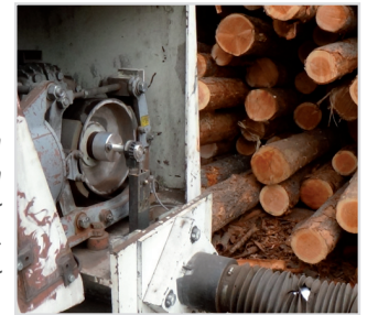
A Model 25T with an FJ Flex Mount Arm mounted on a motor shaft (inspection panel removed). In its harsh outdoor environment at a lumber mill, the dust-tight IP66 seal also protects the encoder from outdoor moisture.
