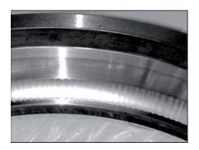
surface material is heated to temperatures ranging from tempering to melting levels. This leads to the appearance of discolored areas, varying in size, where the material has been tempered, re-hardened or melted. Small craters also form on the bearing surface where the metal has melted.
