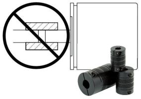
Also, with shaft encoders, it is important to utilize a flexible shaft coupling. Rigid couplings can transmit harmful inputs to the encoder shaft and the bearings such as vibration, shaft end run-out, misalignment or other loads. BEPC offers a number of industry standard Shaft Couplings as accessories. For more complete details on proper encoder installation, see our Encoder Wiring and Installation Guide.
