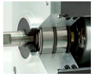
Be aware that there are 3 points of ingress into the encoder: the connector, the shaft or bore, and the bearing hub/case interface. Seal failure in any of these three locations can lead to encoder failure. Be sure that the manufacturers IP rating applies to the entirety of the encoder, as some companies advertise the IP rating of the connector as the rating of the encoder itself.
