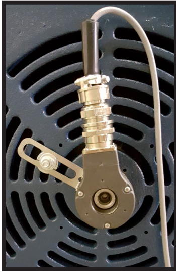
An BEPC Thru-Bore Encoder in a common application, mounted on a motor with an FJ Flex Mount
