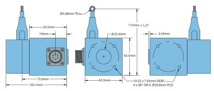
All dimensions are in mm with a tolerance of ±0.127 or ±0.254 unless otherwise specified
