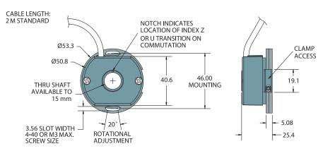
All dimensions are in mm with a tolerance of  $\pm 0.127$  or  $\pm 0.254$  unless otherwise specified.
