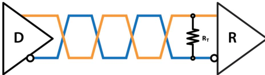
It is usually better to select a value for  $R_T$  that is slightly larger (up to 10% larger) than  $Z_0$ , as over-termination tends to improve signal quality better than under-termination.
