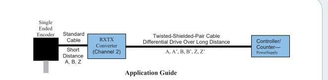
The illustration above utilizes Channel 2 of an RXTX Converter to convert the encoder's single-ended signals (open collector, pull-up, or push-pull) to complimentary-differential signals (which are recommended for signal transmission over long distances).
