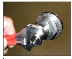
An adjustable wrench or end wrench can be used in the shaft notch to provide additional control for installation and removal
