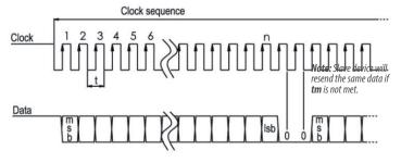
The encoder data bits are sent MSB to LSB, with multi-turn position bits sent first (if applicable), followed by single-turn position bits.
