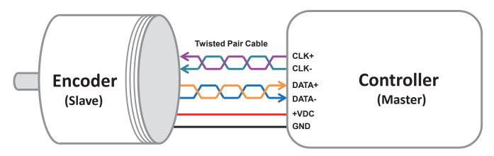
The SSI Master controls the data flow from the encoder data output by sending clock sequences to the encoder clock inputs. The encoder electronics respond to the first falling slope of the clock sequence by freezing the current position value and starting the serial output of the data bits. On every following rising clock edge from the master, one data bit is transmitted by the encoder.
