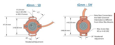
All dimensions are in mm with a tolerance of  $\pm 0.127$  or  $\pm 0.254$  unless otherwise specified.
