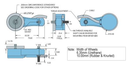
All dimensions are in mm with a tolerance of ±0.127mm or ±0.254 unless otherwise specified
