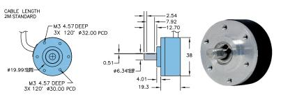
All dimensions are in mm with a tolerance of  $\pm 0.127$ mm or  $\pm 0.254$  unless otherwise specified
