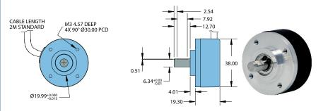
All dimensions are in mm with a tolerance of  $\pm 0.127$ mm or  $\pm 0.254$  unless otherwise specified
