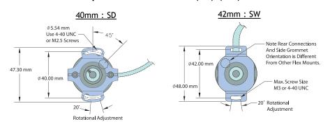
All dimensions are in mm with a tolerance of ±0.127 or ±0.254 unless otherwise specified.
