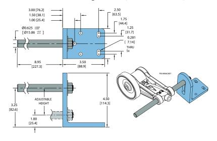
All dimensions are in mm with a tolerance of  $\pm 0.127$ mm or  $\pm 0.254$  unless otherwise specified
